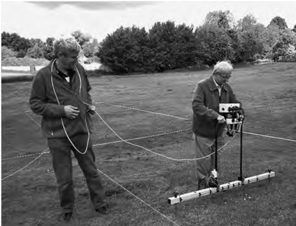
Taking measurements with the resistivity meter
